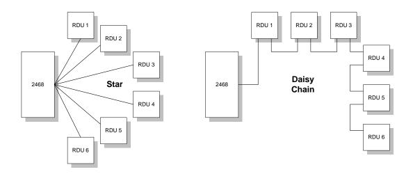
Figure 4.3 - Star and daisy chain connections of remote displays
